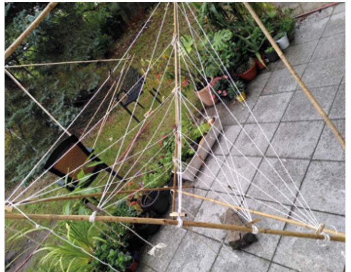
Intermediate position during tensioning: Clothes pegs hold the strings in position.
